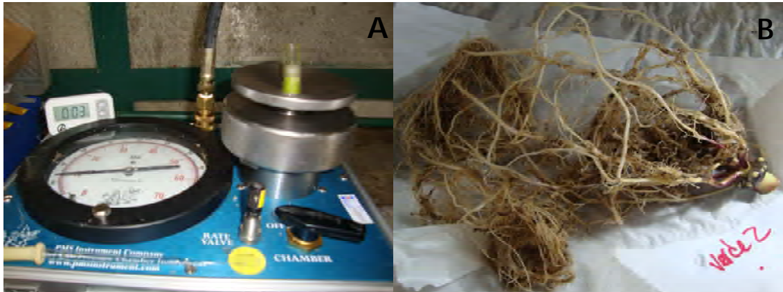
Figure 4: A) Root conductivity measurement with a pressure chamber. B) Shoots excised above the crown of the roots in Venezuelan maize varieties.
