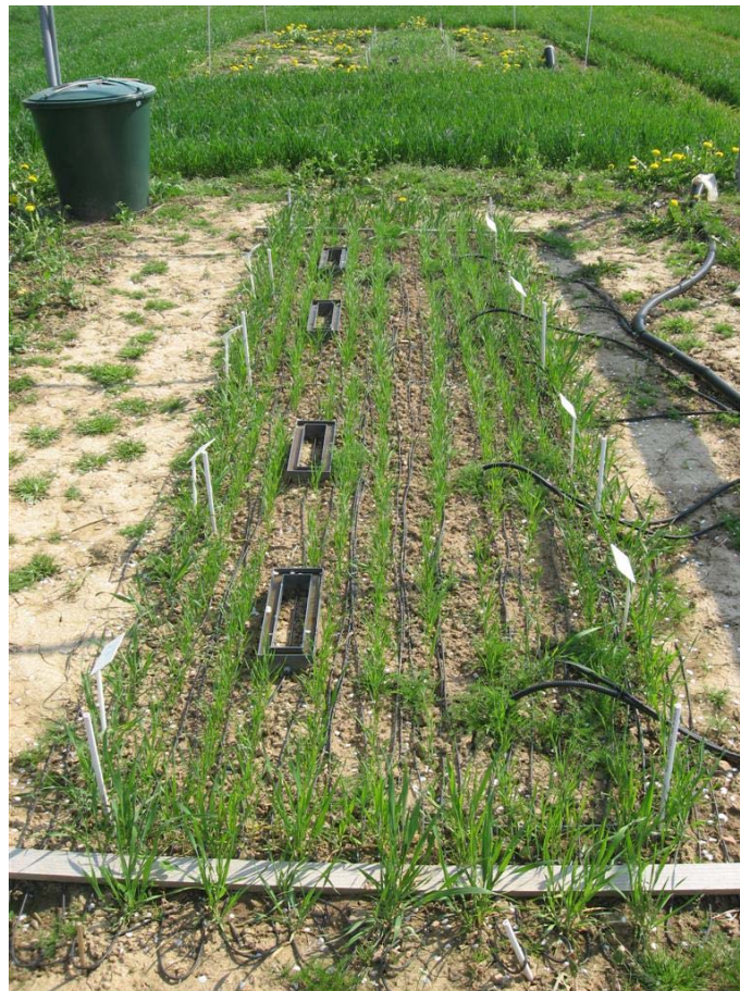
Figure 1; Plot design with soil heating system and control thermometers (picture from Christian Poll)
