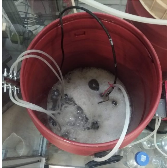
Figure 12: Nitrate-Reactor. Visible aeration hoses connected to aeration plates.
