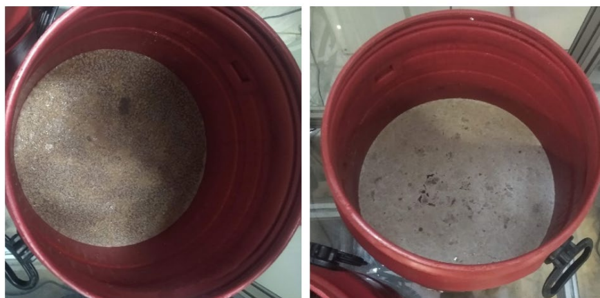
Figure 37: Potassium Reactor on day of experiment 7 (left) and 75 (right) with visible mold formation.
