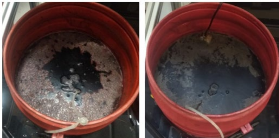
Figure 23: Pictures of Ammonium-Reactor I on day of experiment 7 (left) and day 36 (right), with visible film on the surface.
