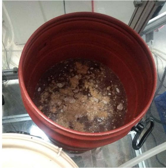
Figure 14: K-Reactor on day of experiment zero. After adding 1992 g of dried and ground potato peel and pulp.
