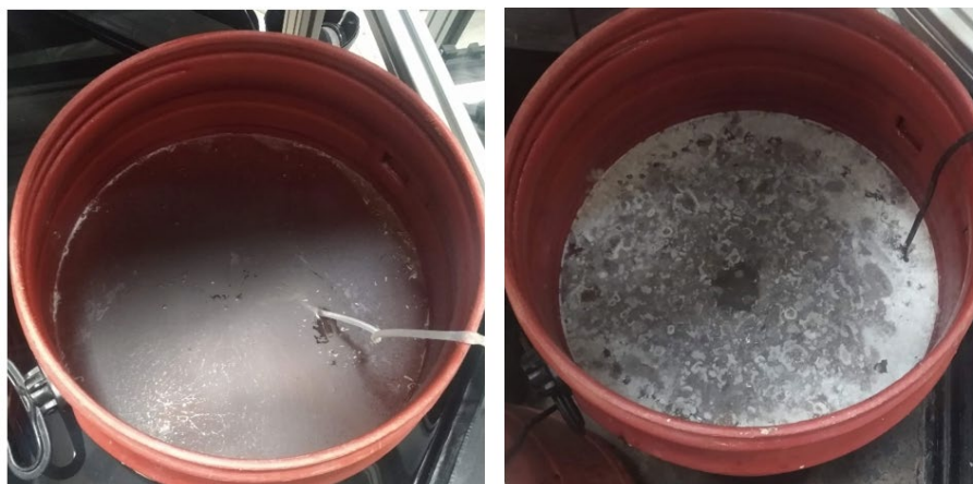
Figure 32: Phosphorus Reactor on day of experiment 7 (left) and 75 (right) with visible mold formation.
