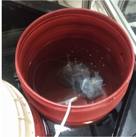
Figure 13: P-Reactor on day of experiment zero. After the addition of bone meal in mash bags.
