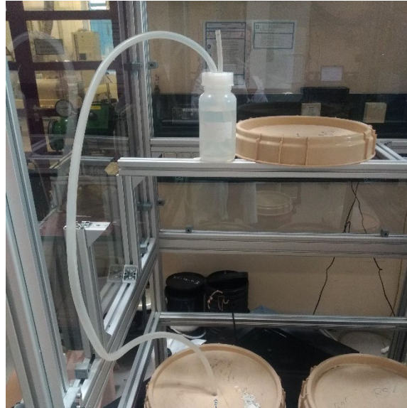
Figure 10: Gas-wash bottle installed to create anaerobic conditions.
