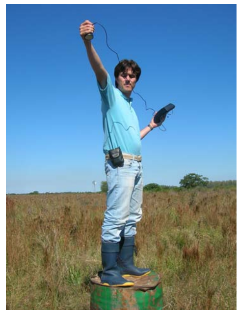
Plate 3.2 In situ determination of NDVI
